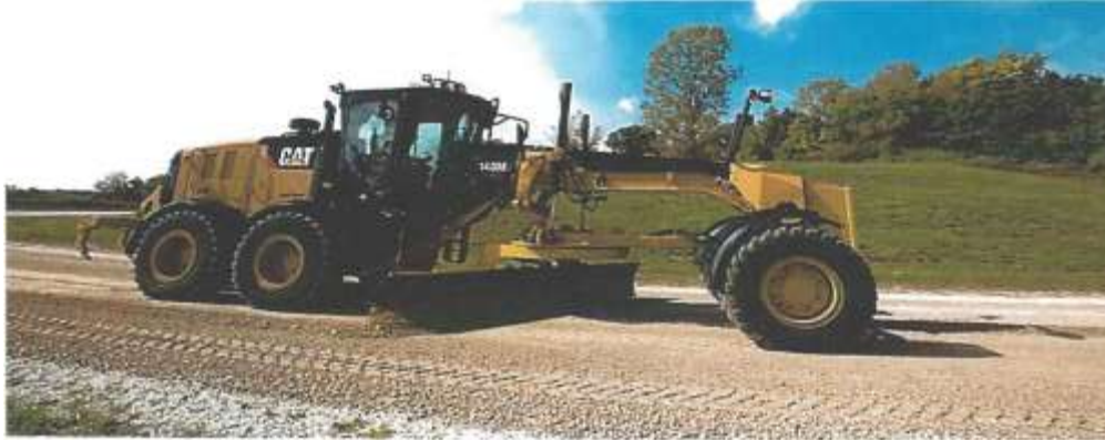
Road Grader: For scarifying roadbed, blade mixing and achieving final grade
