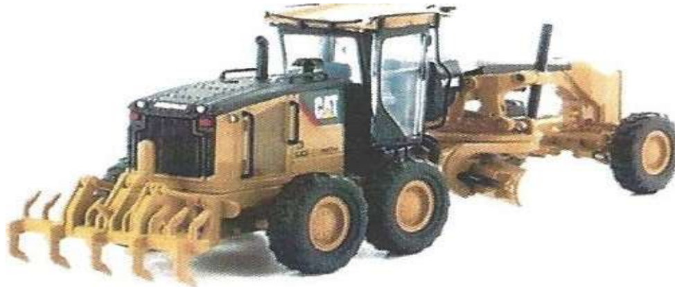
Road Grader: For scarifying roadbed, blade mixing and achieving final grade
